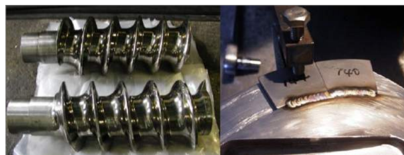
Fig. 24 Weldable WC/Ni FGMs tile and the FGMs screw product for the extruding machine
