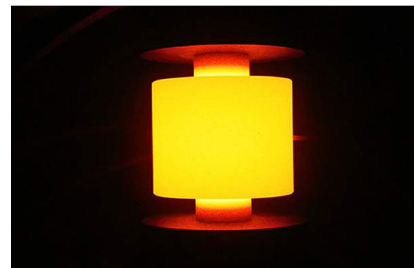
Fig. 6 The sintering stage in a graphite mould and vacuum chamber
