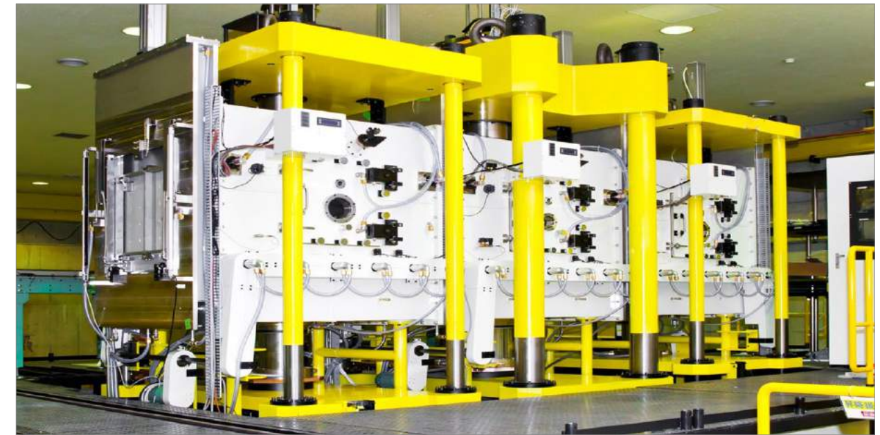
Fig. 9 World's largest semi-tunnel type automatic SPS production system has three vacuum chambers, 6 MN press with a pallet-type special conveyer, and inverter-type 40,000 A DC pulse generator (Courtesy Sinter Land)
