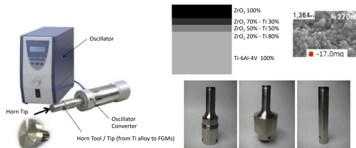
Fig. 14 Ultrasonic homogeniser and ZrO_2 /Ti alloy system FGM horn tip tool (manufactured by Mitsui Electric Co.,Ltd, Japan)
